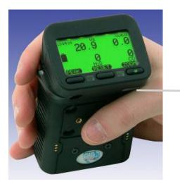
Turn the G460 on in an environment known to be free from gases and / or vapors.
