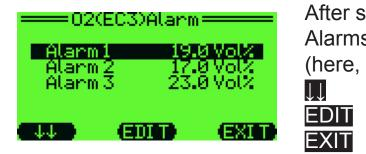
After selecting the sensor menu point Alarms the following reading is displayed (here, for an  $O_2$  sensor):
