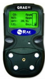
This compact portable device monitors up to four gases in confined spaces.
