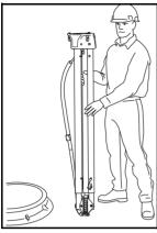
(1) Tilt the Workman Tripod into an upright, feet-down position.
