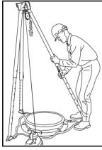
(5) Raise the Workman Tripod one leg at a time by pulling the pin (attached to the upper leg section), incrementally sliding out the lower leg section, and repinning. Repeat for each leg until the Workman Tripod head is at the desired height. The Workman Tripod head should be level when installation is complete. Be careful not to extend each leg too far in each increment so as to cause the Workman Tripod to topple.
