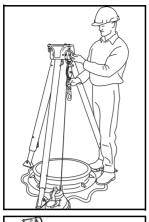
(4) Optional components to be attached to the Workman Tripod Head, such as the Split-Mount Pulley, should be assembled to the Workman Tripod Head at this time. Follow the appropriate user instructions for each optional component that is to be connected to the Workman Tripod.
