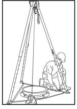
(6) Once at the proper height, check to be sure the Workman Tripod is stabilized and plumb.
