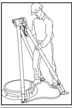
(2) Hinge each leg, one at a time, into the outward and locked position. Note that each leg automatically snaps upward when the hinge locks. Check to be certain of hinge locking.
