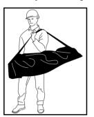
The Nylon tote bag is used to protect the Workman Tripod during transport and storage.
