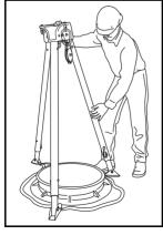
(3) Position the feet about the hatch cover in accordance with work area geometry and surface conditions.
