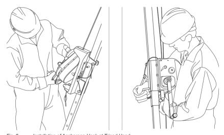
Fig. 8 Installation of Anchorage Hook at Tripod Head
