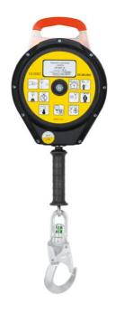
Retractable type fall arrester CR 200 in plastic cover with expandable steel cable. The device is intended for works requiring significant mobility in respect to attachment point. Energy absorber is not required. Retractable type fall arrester CR 200 is a component of personal fall protection equipment. The device is tested and approved for working on flat roofs in combination with roof lanyard AZ 800.
