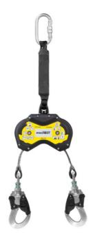
DWR040S is a lightweight fall arrest device with two webbings, designed for work requiring frequent changes of the attachment point. The locking mechanism is located in a durable housing with a swivel in the upper part of the device. No need for an additional safety shock absorber. The device has built-in snap connectors AZ 001ASI or AZ 029SI with a swivel and an indicator.
