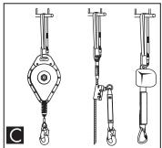
The structural anchor point should be situated above the working place and the shape of the structural anchor point should not let self-acting disconection of the Webbing Sling Connector.
