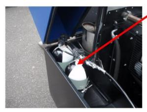
BACKUP EMERGENCY SUPPLY CYLINDERS LOCATED AT THE SIDES OF MAIN COMPRESSOR HOUSING
