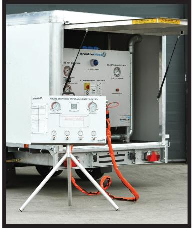
Thermac has developed the UK's first unit that combines both precision dustless shot blasting equipment and a breathing air compressor into a single road-towable, enclosed trailer.
