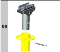
Insert the A5032-07 winch support into the post and insert the pin in the hole to secure it.
