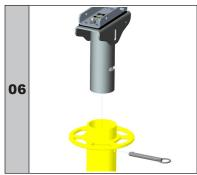
Insert the A5032-07 winch support into the post and insert the pin in the hole to secure it.
