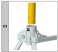
Insert the A5032-01 post into A5032-15 and ensure that the pin holes are aligned.
