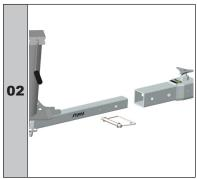
Insert part IN-2517 into the end of A5032-15.
