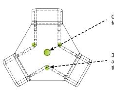
Central anchor point for pulley.
