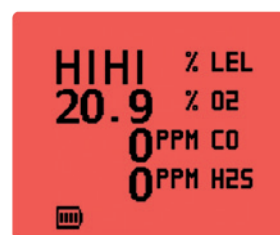
Red display in alarm conditions
